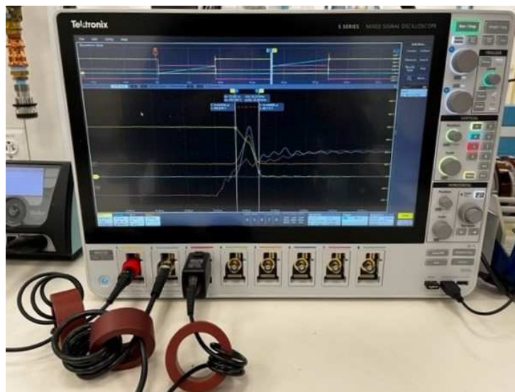
Figure 35: Oscilloscope Shown with Nanocrystalline Common Mode Cores
