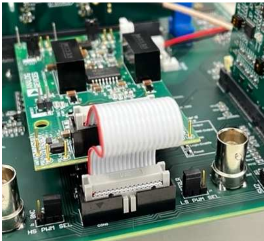
Figure 19: Jumper set to CTRLR input
