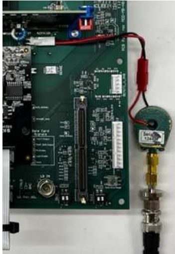
Figure 28: High-Bandwidth CT Connected to CON11
