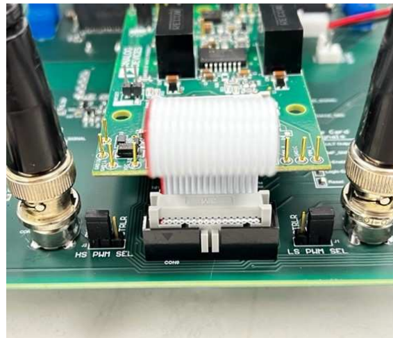
Figure 20: Jumper set to BNC input
