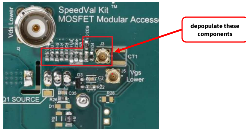
Figure 26: Daughter Card with Shunt Resistors
